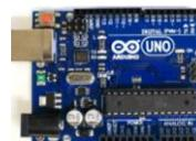
Gambar 1.5 Board Arduino Uno
